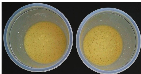
Fig. 1 - Visually similar grainy texture in two samples after homogenizing and subjecting it to the isothermal experiment at 26 °C with seeding
