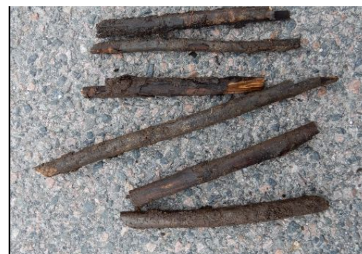
Fig. 1 – Wood twigs with diameters of 10-15 mm taken from a garden compost.
